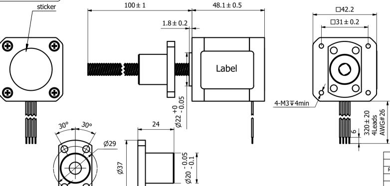
Motor's phase 2 Step angle 1.8° Rated current/phase 2.5 A 1.0Ω±10% Resistance/phase Inductance/phase 1.8mH±20% 0.01mm/step Linear travel per step Ball screw diameter Ф8.0mm Ball screw lead 2.0mm C7(KSS) Grade Insulation class В 100MΩ(500VDC) Insulation resistance 80°C Heat rise 0.386 kg Motor weight
