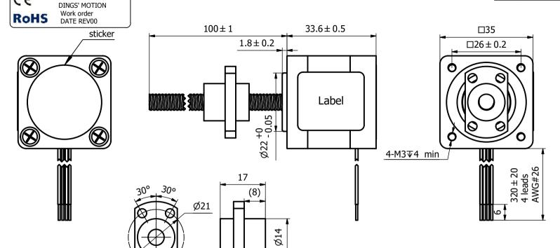
Motor's phase 2 Step angle 1.8° Rated current/phase 1.0 A 3.5Ω±10% Resistance/phase 3.6mH±20% Inductance/phase 0.03mm/step Linear travel per step Ball screw diameter Ф6.0mm 6.0mm Ball screw lead C7(KSS) Grade Insulation class 100MΩ(500VDC) Insulation resistance 80°C Heat rise 0.18 kg Motor weight
