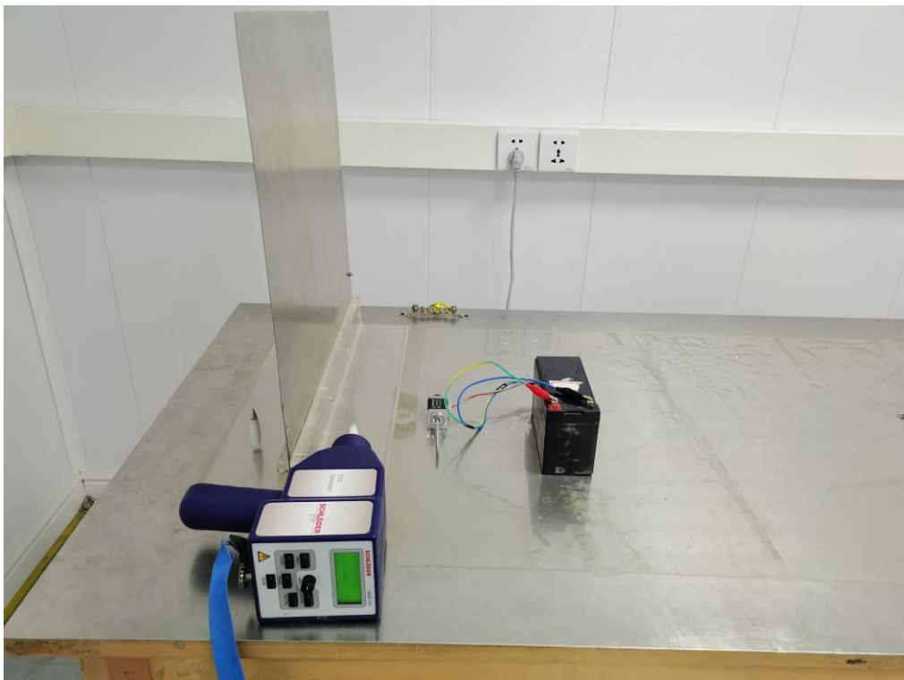
Test Setup Photo of Electrostatic Discharge Test
