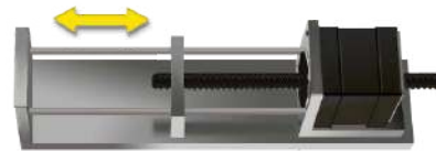
Non-Captive Lead Screw Linear Actuator + Guided Rod
