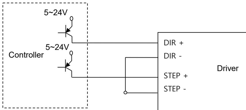
**3.2 Input Signal of Switch or Relay Connection**
